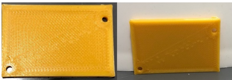
Figure 9. Manufactured Battery Door
