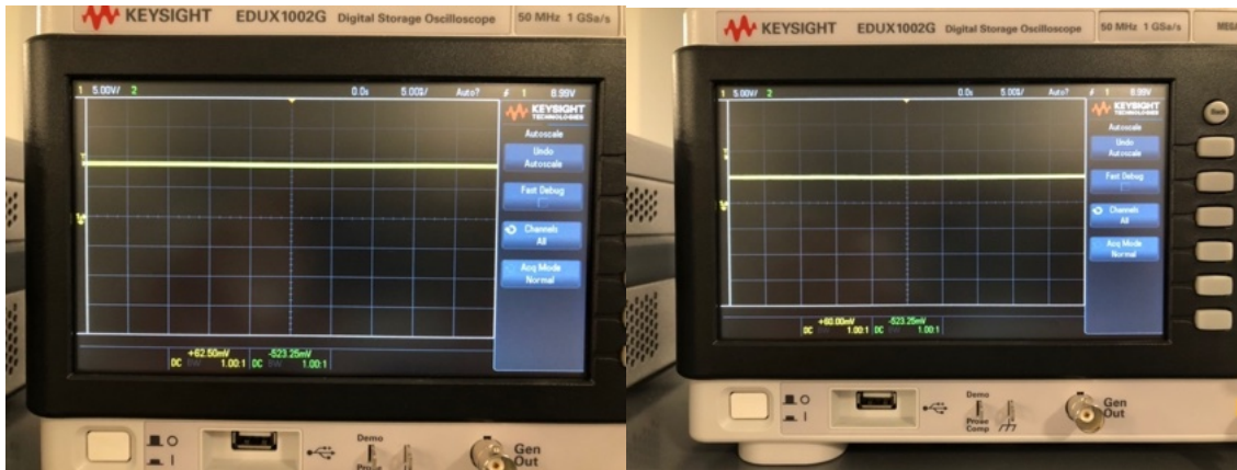
Figure 15. Confirmation of Battery and Voltage Regulator Output
